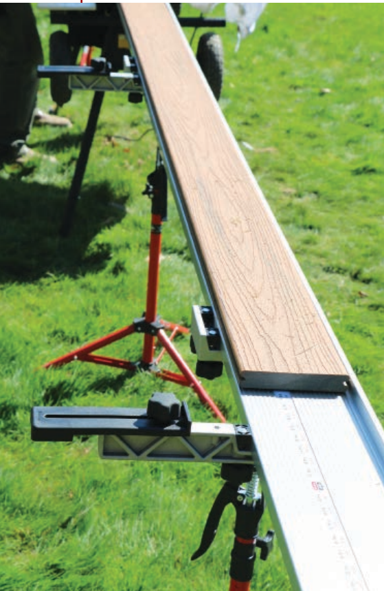
Figure 2. FastCap's optional molding stop, used here to help keep the decking from sliding off the fence.
