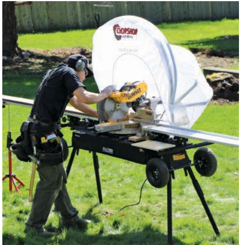
Figure 3. The optional chop saw hood contains dust and can be used to help keep the saw dry in wet weather.
